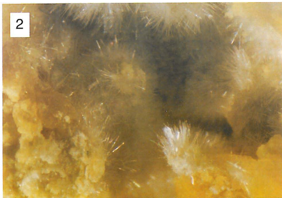
1 — Growths of fibrous pickeringite with silky luster, \times 10 2 — Acicular pickeringite on yellow copiapite, \times 15
